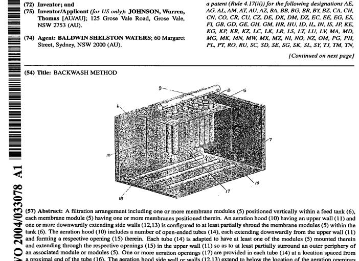
an associated module or modules (5). One or more aeration openings (17) are provided in each tube (14) at a location spaced from a proximal end of the tube (16). The aeration hood side wall or walls (12,13) extend to below the location of the aeration openings (17) in the tubes (14). Gas providing means (18) feed gas into the hood (10).
